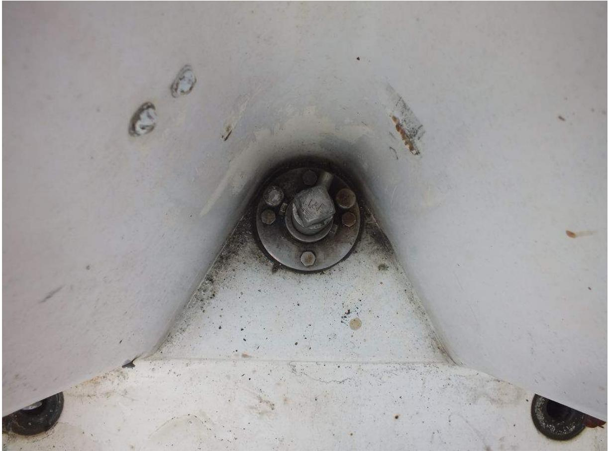
**REMONTAGE ET CHANGEMENT DES BAGUES DE SAFRAN AVEC PALIER EN ELASTOMERE AUTO-ALIGNANT**
